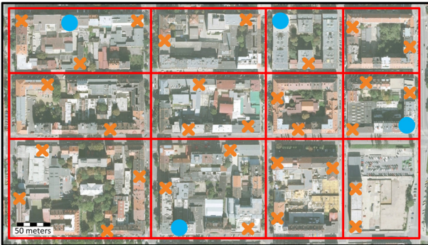
Fig. 6. Environment for simulation with depicted position of MeNBs (blue circle) and SCeNBs (orange cross).
