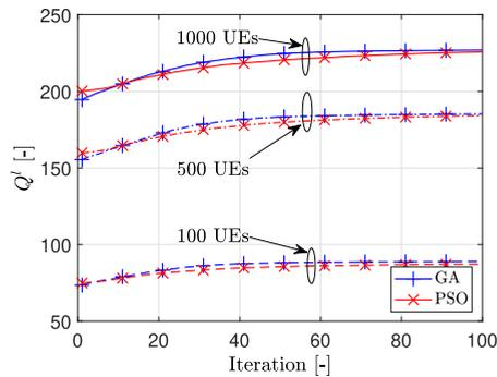
**FIGURE 7. Evolution of cost over iterations of the GA and PSO for  $C_{\min}^{\min} = 10$  Mbit/s.**
