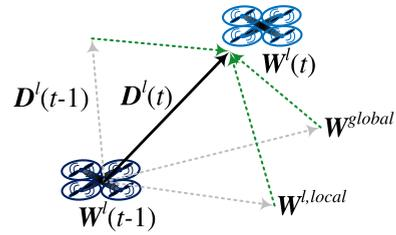
**FIGURE 1.** Update of FlyBS position via the proposed algorithm based on PSO.
