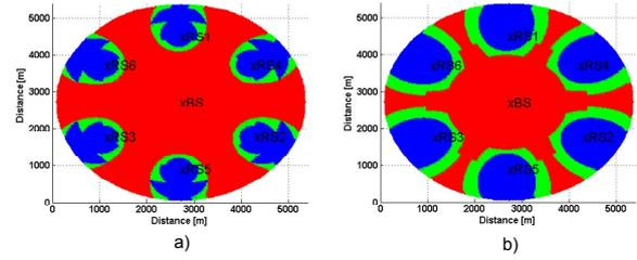
Fig. 9. Association when reuse of RSs resources is enabled
