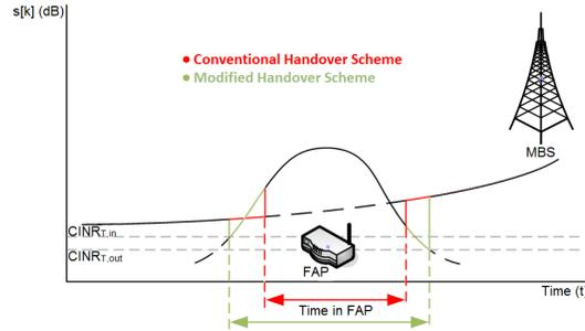
**Fig. 1.** The principle of the modified handover schemes.
